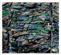
**Piles of old plastic** PET recycling starts with sorting and squashing bottles into huge bales. These are sent to a recycling plant, where machines grind them into tiny flakes. After washing, the flakes are sold on to plastics factories.
