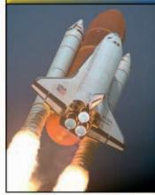
Rockets work because they follow Isaac Newton's third law of motion: each force (an action) has an equal force in the opposite direction (the reaction). As the fuel burns, the expanding exhaust gases are pushed backward, and the Newtonian reaction pushes the rocket forward. Saturn V rockets took off from Launch Complex 39
