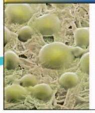
The glue contains billions of tiny sticky acrylic spheres; the gaps between the spheres prevent them from sticking too well. A coating on the back of the notes makes the glue stay on them and not transfer to the other surface.
