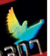
Holograms are pictures that appear in 3-D (threedimensional). Making a hologram involves lasers, beam splitters, lenses, mirrors, and special film. Holograms make it very difficult to produce fake copies of credit cards.
