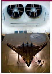
The X-48B Boeing Phantom is a type of experimental plane based on a flying wing design. This means that the entire plane is designed to act as a single huge wing, all of which provides an upward thrust on the plane. However, the shape of these experimental planes makes them difficult for pilots to control.
