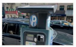
**Cheaper meters** Parking meters are sometimes fitted with solar cells. This is because they are used outside where there is plenty of sunlight and need very little electricity to operate.
