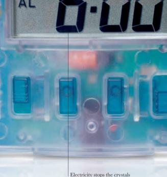
Electricity stops the crystals from letting light through the glass, so these areas are dark
