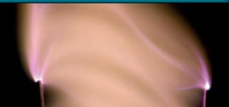
Edison and Swan built upon decades of research to use electricity to make light. Sir Humphrey Davy made a key breakthrough in 1809. He found that an arc of electricity jumps between two carbon sticks to complete a circuit, heating the carbon until it glows.
