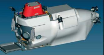
The Wood's Hole Oceanographic Institute in the U.S.A. is building a new submersible. It will be able to dive deeper than their existing submersibles and stay on the seabed for longer. It will also have more room inside for the crew.
