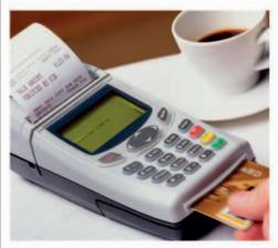
**Chip and pin machine** In restaurants and cafés in many parts of the world a small wireless chip and pin machine is taken to the customer. The credit or debit card is inserted into the device and the transaction is authorized by the customer's personal identification number (PIN). This payment method is quick and secure.
