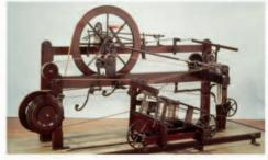
**Crompton's mule, 1779** The next significant improvement was Samuel Crompton's spinning mule; it could make many types of threads quickly and easily.
