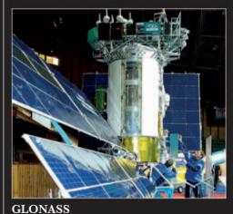
Russia completed its own satellite navigation system, called GLONASS (Global Navigation Satellite System), in 1995. The GLONASS satellites orbit at a height of 11,868 miles (19,100 km), a little lower than GPS satellites.
