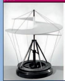
The concept of flight fascinated Italian artist Leonardo da Vinci. More than 500 years ago, he designed a flight machine that resembled a helicopter. Although not practical, Leonardo's design was way ahead of its time. This modern model is based on Leonardo's drawing. The rotating wings, (blades) are shaped to provide maximum lift as they turn -
