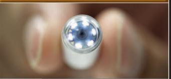
An endoscope the size of a large pill has been developed. Called a capsule endoscope, it is swallowed by a patient and passes through the body, transmitting pictures on its way. Future capsule endoscopes may be self-propelled and able to carry out minor surgery using a movable arm.
