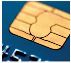
**Smart card chips** The chip is a microprocessor: it can handle digital information, just like a tiny computer. Card readers usually need a personal identification number (PIN) to access this personal information. This system is widely used in Europe.
