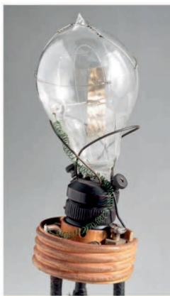
**Thermionic valve** These were vacuum tubes that could change or halt the flow of electricity. They contained small heaters and glowed like lightbulbs. This is a very early one.
