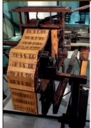
Like a robot, the Jacquard loom followed coded instructions, but while modern robots receive instructions from computers, the loom was controlled by cards with holes punched in them. These directed the positions of the threads, so different patterns could be woven automatically. It was invented in 1801 by Joseph-Marie Jacquard.
