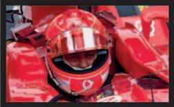
**Built for speed** The helmets worn by Formula 1 racing drivers are individually made for each person. A helmet is made of at least 17 layers of materials such as carbon fiber.
