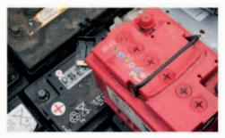
Lead-acid Cars use lead-acid batteries. Although heavy, they are very powerful and can be recharged by the car's engine.
