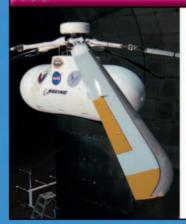
Helicopters use a lot of fuel. They also make a lot of noise. Scientists, however, are developing new types of helicopter blades that change shape when electrical signals are fed to them. This makes them move through the air more quietly, and means less fuel is needed, too.
