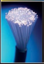
When light enters one end of an optical fiber, it stays inside the fiber. Even if the fiber is bent or tied in a knot, the light stays inside it and follows it to the end, like water flowing through a bent pipe. Optical fibers have to be made of very pure glass, free from defects, in order to carry the maximum light intensity from end to end.
