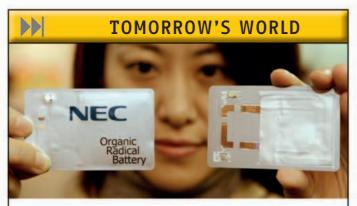
These organic radical batteries are bendable, less than <sup>1</sup>/<sub>25</sub> in (1 mm) thick, and are fully charged in less than 30 seconds. They do not use harmful metal chemicals to make electricity, so they can be safely thrown away.
