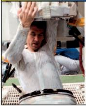
Here on Earth, we keep cool by sweating. Sweating doesn't work inside a spacesuit. Instead, an astronaut wears a layer of underwear with a plastic tube sewn into it. Cool water flows through the tubing and carries heat away.
