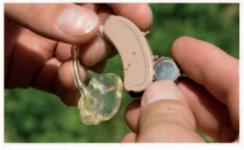
Zinc-air Tiny zinc-air batteries are used to provide the power for hearing aids. They need oxygen from the air in order to work.
