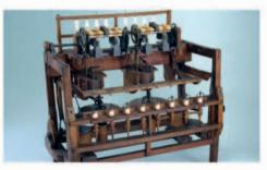
Arkwright's water frame, 1768 Richard Arkwright's invention was an important improvement on the spinning jenny. It made stronger cotton threads, and was powered by a water mill.
