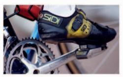
**Cycling shoe** Many cycling shoes have clips, which are also called cleats, on their bases. Cleats can be slotted into bicycle pedals to stop the shoes from slipping.
