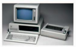
**IBM 5150, 1981** The IBM Personal Computer was very popular, and other manufacturers soon built similar machines, with separate keyboards, monitors, base units, and printers.
