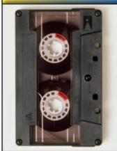
A cassette contains plastic tape with magnetically charged particles. The tape passes over a playing head, which reacts with the magnetic particles. This creates vibrations that are converted into sound by the headphone speakers.
