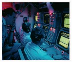
**Taking control** Submariners command the vessel from a control room below the sail, sitting in front of an array of computer screens and instruments. Most of the controls for navigating, diving, and fighting are here.
