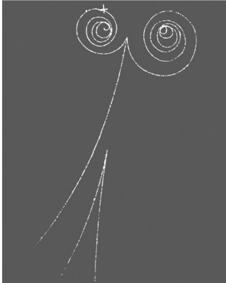
27. Pair production: matter and antimatter are created directly from the energy of a photon. A gamma ray photon enters from the top, passes close to an atomic nucleus, and produces an electron (left-handed spiral), and a positron (right-handed spiral). A recoiling atomic electron emerges downwards.
